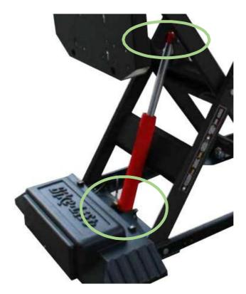
Figure 12 — hydraulic piston
