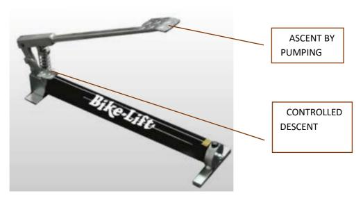
The operation is very simple: press the foot pedal repeatedly, making it move alternately from top to bottom to generate hydraulic pressure. By stopping the action on the pedal, the pump will stop but will remain under pressure.
