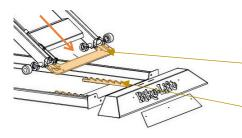
mobile anchoring bar with automatic coupling that prevents the accidental descent of the mobile surface.
