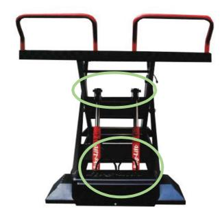
Figure 8 - hydraulic pistons
