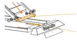
a mobile anchoring bar with automatic coupling that prevents the accidental descent of the mobile surface.
