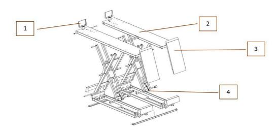
Figure 6 — general model of a lifting platform
