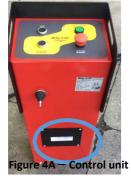
The operations of ascent/descent, safety release and immediate stop in case of an emergency are carried out by means of the lifting platform control unit (Figure 4A).
