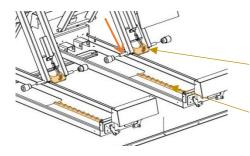
mobile anchoring bar with automatic coupling that prevents the accidental descent of the mobile surface.
