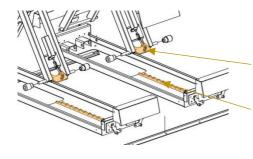
a mobile anchoring bar with automatic coupling that prevents the accidental descent of the mobile surface.
